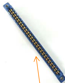
Edge finger of probe card slides into the edge connector. The connector is mounted to the probe card holder's adjustable rails
